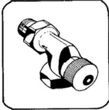
6. Tighten metal collar on control to valve body, orienting white triangle on control base so that it is in view. Metal collar may be locked using set screw on side.
