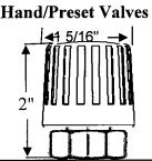
The American Steam Control manual hand valves are combination shut off and union valves for steam and hot water applications.
